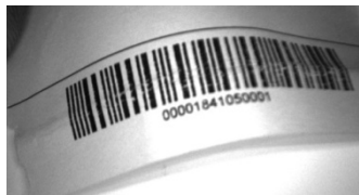
Figure 20 - Barcode Printed on Curved Surface Readable by Matrix 300N in spite of Image Optical Distortion
