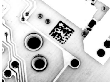
Figure 25 - Data Matrix Code Directly Marked on PCB Surface by Using Laser Etching Technology
