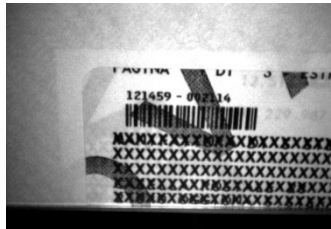
Figure 19 - Overprinted Barcode Readable by Matrix 320 also Through the Envelope Window Film
