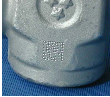
Figure 21 - Dot Matrix Code Directly Marked on Metal Surface by Using Dot Peening Technology
