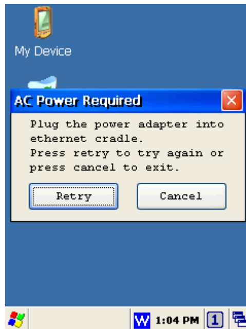
FIGURE 3-63 AC POWER REQUIRED
