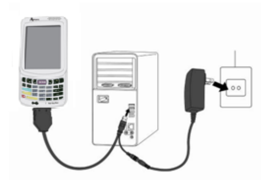
Figure 2-14 Communication through Cable
