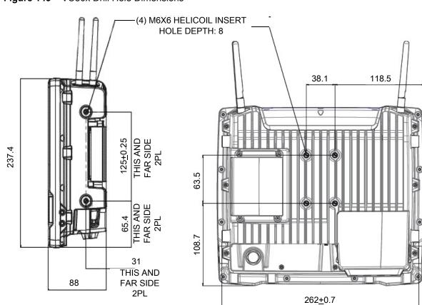
Figure 143 VC80x Drill Hole Dimensions
