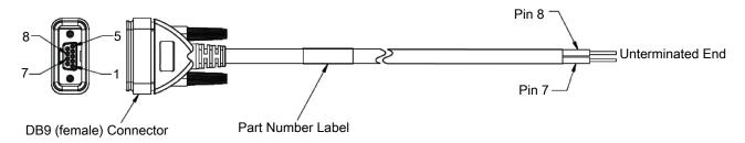
Figure 14 Screen Blanking DB9 Pin Configuration
