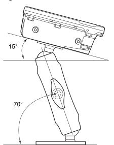
Figure 87 Orientation of Vehicle-Mount Assembly
