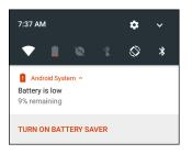
When the battery charge drops below 15%, the VC80x displays a notice to connect the VC80x to power. The user must charge the battery using one of the charging accessories.
