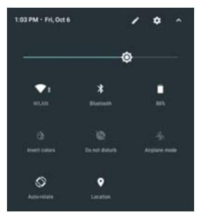
2. Touch WLAN to open the WLAN screen. The VC80x searches for WLANs in the area and lists them.
