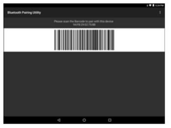
Using the RS507/RS507x/RS6000, scan the barcode on the screen or scan the barcode on the right side of the VC80x.
