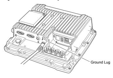
**CAUTION** Attach the VC80x connecting cable as close to the battery as possible. Connecting the VC80x to large electrical loads, such as converters for the forklift motor may result in random restarts, malfunctions and/or irreparable damage to the device.
