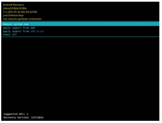
10. Press the Volume Up and Volume Down buttons to navigate to apply from USB drive.
