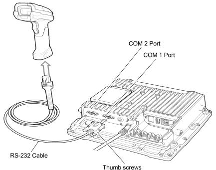
Figure 69 Connect RS-232 Scanner
