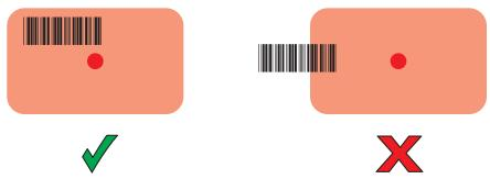
Figure 68 DS3678-SR Pick List Mode with Multiple Bar Codes in Aiming Pattern
