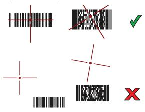
Figure 65 Pick List Mode with Multiple barcodes in Aiming Pattern
