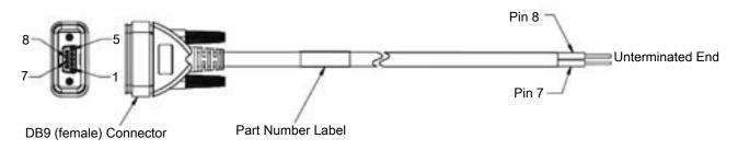
Figure 13 Screen Blanking DB9 Pin Configuration
